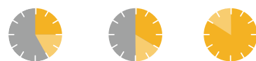
3 to 5 hours recovery time = 15 amps per bank 4 to 6 hours recovery time = 10 amps per bank 10 to 12 hours recovery time = 5 or 6 amps per bank
